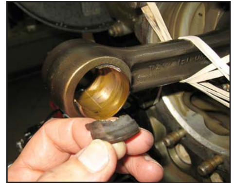
Above: Broken bushing on a 421C. Large pieces like this are usually found in the oil sump. Left: Picture from CSB07-01A.
